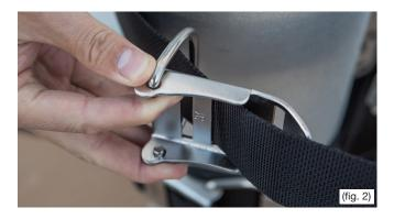
Make a U-turn and pass the webbing through the slot closest to the wire bail (fig. 3).
